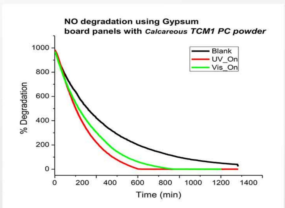
Lower concentration of NOx oxides in the Demo Houses which were painted with PC paint
